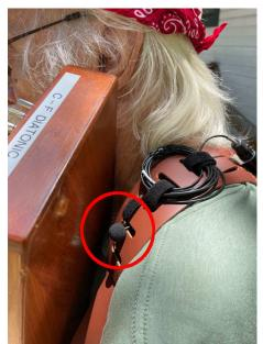
The B3 comes in two sensitivities, normal and low. With a bit of measurement, I found that that the maximum sound level at the back of a good autoharp is about 95 dB, and the normal sensitivity B3 seems to be quit adequate.
